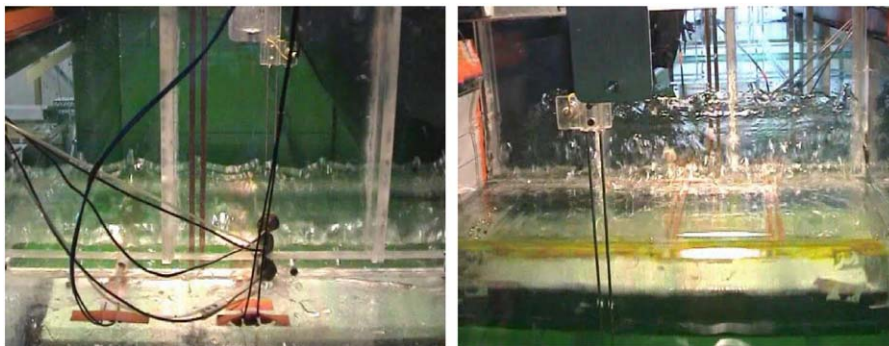
Fig. 19. Three-dimensional instabilities of the water front during the run up after the impact. Left: back view. Right: front view.
