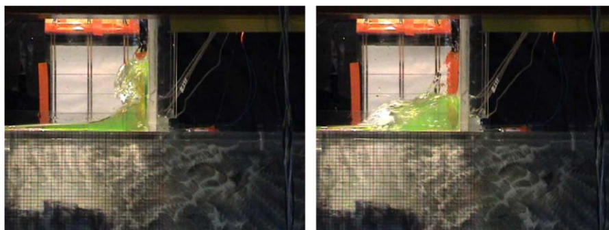
Fig. 7. Two-dimensional laboratory experiments ( \lambda/D = 10.1 , H/D = 0.808 ): late evolution of the impact against the vertical superstructure. After the maximum run-up the water plunges backward onto the deck.
