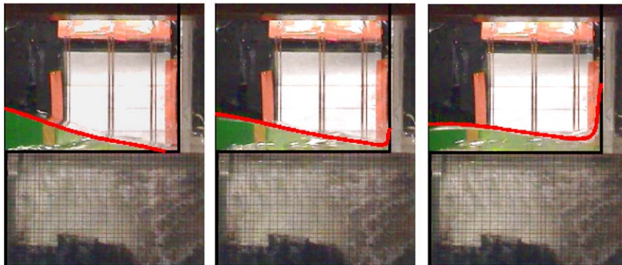
Fig. 16. Impact of the shipped water against a vertical superstructure located at 0.2275 m from the model bow. Water shipping is induced by waves with \lambda/D = 10.1 and H/D = 0.808 . Red lines are the present numerical simulations. Time increases from left to right: time instants from the water shipping starting \Delta t_{\text{wod}} = 0.273 , 0.313 and 0.353 s (2.603, 2.984 and 3.366 s full-scale draft D = 18 m).
